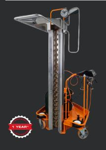
The Turbopack is a mobile heating column, loaded on an easily movable trolley. It gives the operator the possibility to heat-shrink his load anywhere in the shipping area, very useful to avoid the movement of unstable loads.
